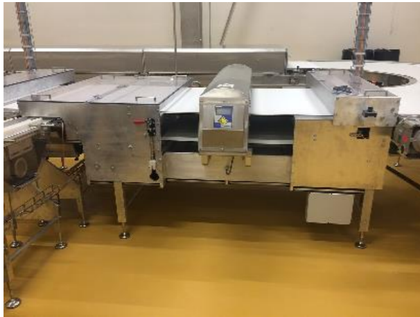
Conveyer with metal detector, 1 conveyer
